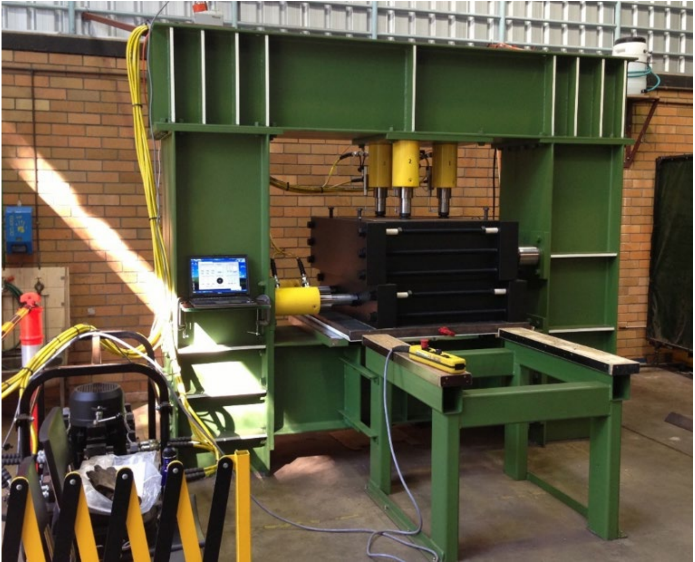
Fig. 6. Photograph of large direct shear machine (LDSM)
